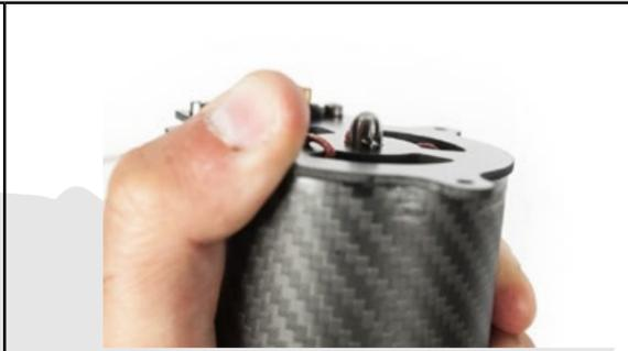
Lock the arming rod with the "Remove Before Flight" pin.
