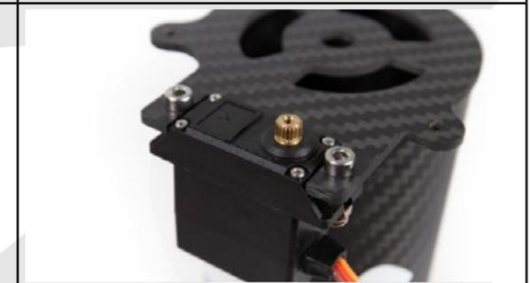
Use the horizontal horn ( the other horns provided with the servomotor won't be used).
