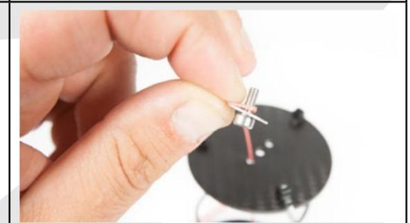
Insert the screw with the line into the piston middle hole.
